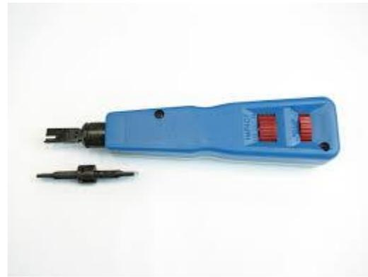
On the left, above is an image of a push down termination patch panel and on the right the associated tool required. The solid core cable is pushed in to the correct position and then small blades within the termination point cut through the conductor's insulation and grip on to the conductor. Secondly solid core cables are far more capable at long distances, stranded cables over long distance can cause degradation in signal quality.
