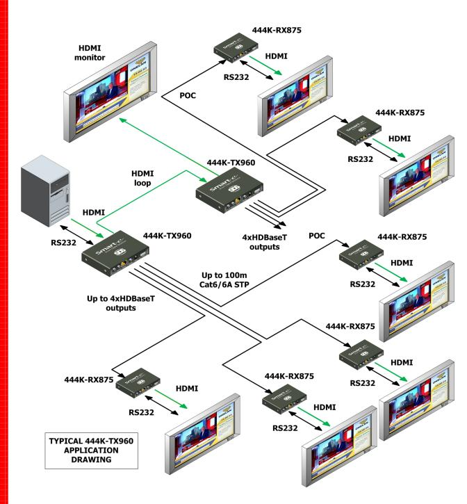
Application showing an 8 display configuration + a local monitor using the looping input feature
