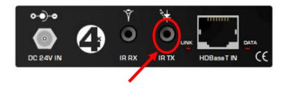
NOTE: Only IR TX units supplied with the 866 unit are compatible, use of other IR TX devices may result in no infra-red functionality.
