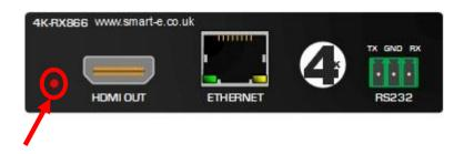
The HDMI hot-plug detect LED is located next to the HDMI socket on both the TX and RX variants of the 866 and is located as indicated above. This LED shows that the 5V, Hot-Plug Detect mechanism of the HDMI is working correctly. A HDMI compliant source outputs a +5V signal, this signal is detected by a HDMI compliant screen and it responds with a Hot-Plug Detect +5V signal to tell the source a screen is attached. The 4K-866 can handle this mechanism at both the TX and RX end.
