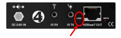
A HDBaseT indicator LED is located next to the RJ45 HDBaseT connector on both the TX and RX variants of the 866. This is the primary indication to show the CATx cable used is suitable to enable the TX and RX devices to communicate with one another. When working this LED should be lit solid red. If not lit or blinking it means, there is a problem with either the transmission medium (CATx cable) or with either the TX or RX unit.
