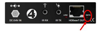
The HDMI data LED is located next to the HDBaseT RJ45 connector as indicated above. This LED shows the flow of HDMI data and the type of HDMI data.
