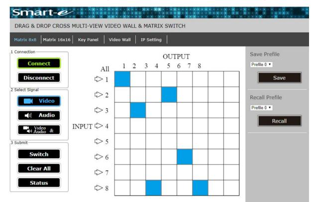
selecting a square on the matrix view and the square will colour blue to indicate a crosspoint selection. Profiles (frequently used configurations) can be saved and recalled at will using the righthand buttons.
