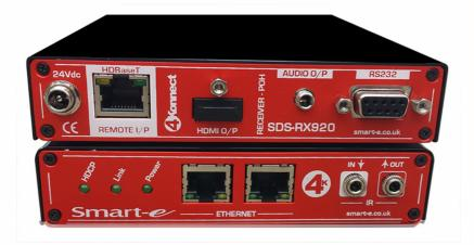
The **SDS-RX920** is a HDBaseT receiver unit designed to accept a Cat 6 input and output a HDMI signal together with bidirectional infrared and RS232 signals over a single twisted pair CAT 5e-8 cable. The units use HDbaseT technology to extend PC resolutions up to 1920x1200 @60Hz together with 1080p @60Hz. In addition the **SDS-RX920** will also deembed the audio within the HDMI transmission.
