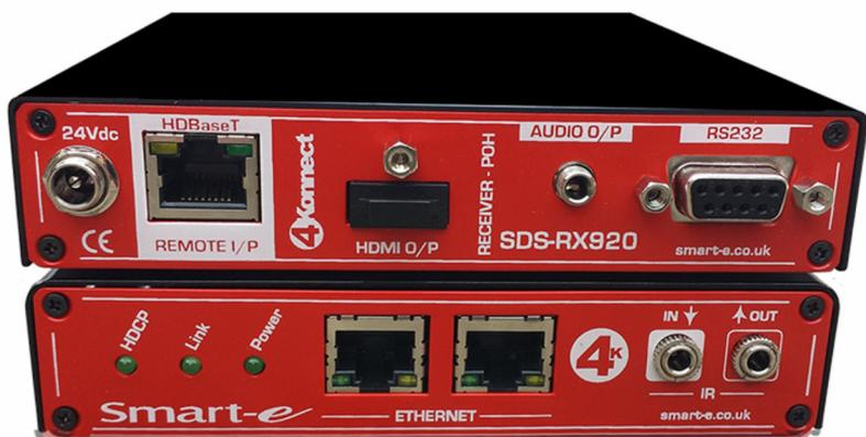
The **SDS-RX920** is a HDBaseT receiver unit designed to accept a Cat 6 input and output a HDMI signal together with bi-directional infrared and RS232 signals over a single twisted pair CAT 5e-8 cable. The units use HDBaseT technology to extend PC resolutions up to 1920x1200 @60Hz together with 1080p @60Hz. In addition the **SDS-RX920** will also de-embed the audio within the HDMI transmission.
