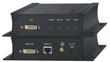
The SDS-922-DVI is a long range extender pair designed to extend DVI-D signals together with reverse IR and bidirectional RS232 signals over a single twisted pair CAT 5e-8 cable. The units use HDbaseT technology to extend PC resolutions up to 1920x1200 @60Hz together with 1080p @60Hz
