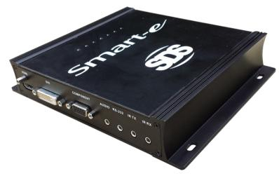
The SDS-TX950 is a multi—function transmitter designed to extend and scale multiple signal types including HDMI, DVI, RGBHV and standard definition analogue video signals together with reverse IR and bidirectional RS232 signals over a single twisted pair CAT 5e-8 cable. The units use HDbaseT technology to extend PC resolutions up to 1920x1200 @60Hz together with 1080p @60Hz
