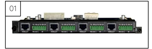
LDX-IP4-HDBT LDX-OP4-HDBT 4 way HDBaseT transmitter and receiver blade
