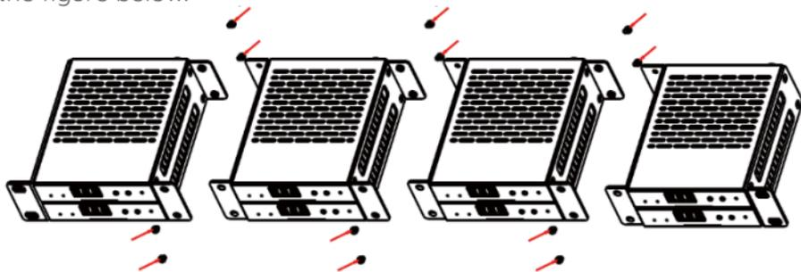
Step 3: Fasten screws between two 1U rack panels, so that eight products are mounted in a 1U rack, as shown in the figure below:
