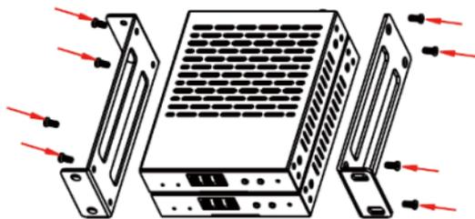
Step 2: Fix two 1U rack panels on another two stacked products in the same way, then use screws to fix two 1U rack panels together, as shown in the figure below:
