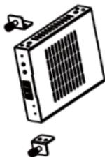
Step 2: Insert the product with mounting ears into a 4U rack (up to 12 units can be installed vertically), as shown in the figure below:
