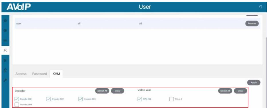
To test KVM access permissions, please plug the mouse and keyboard into the USB Device port of any decoder on the Video Wall KVM\_1X2 used for KVM operations. The screen of the decoder will immediately pop up the KVM login menu, as shown in the following figure.
